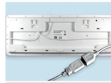
CHOOSE OUT OF 4 CABLE EXIT DIRECTIONS PLUS QUICK DISCONNECT EXTENSION
